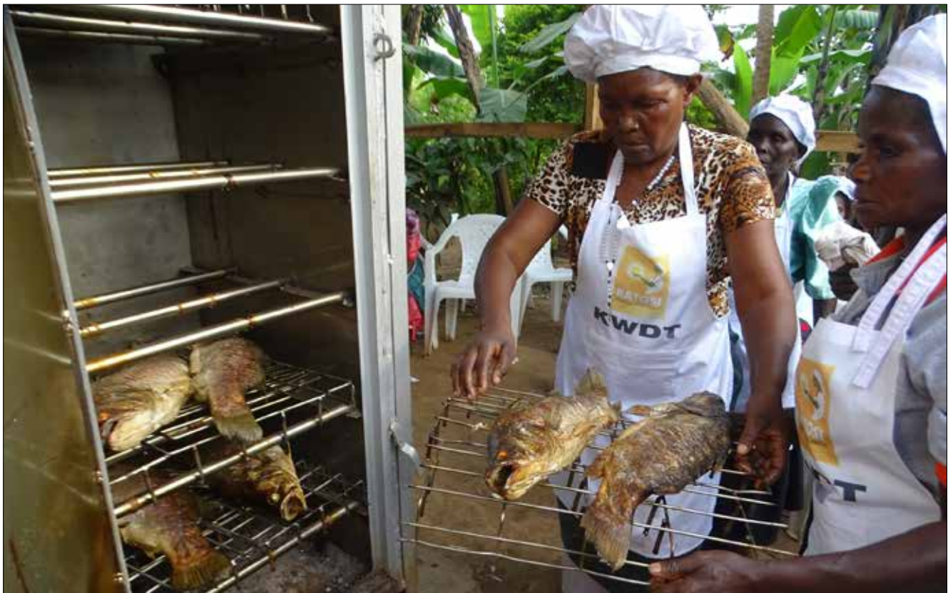
A female fish processor from Bugoye women's group using NARO PAH-Safe fish smoking kiln. The NARO PAH Safe Fish Smoking Kiln reduces smoking time, thus freeing women to attend to other productive roles
