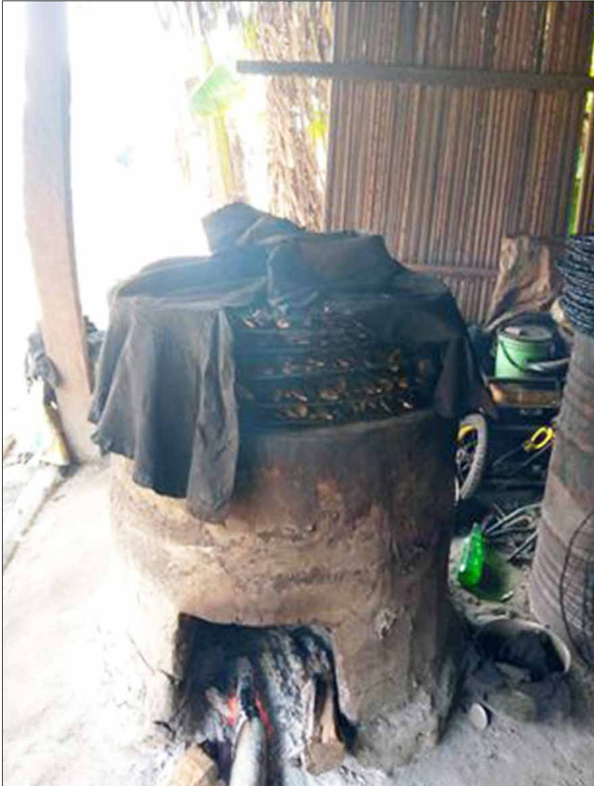
Mud oven with layers of fish trays in Lagos State, Nigeria. Traditional fish-smoking kilns, characterized by fuel inefficiencies, consume more fuelwood than necessary and contribute to forest depletion
